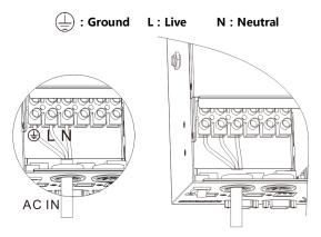
③ Properly connect the AC output wire according to the wire sequence and terminal position shown in the figure below. Please connect the ground wire first, and then the live wire and the neutral wire. The ground wire is connected to the grounding screw hole on the cabinet through the O-type terminal.
