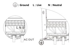
**Note:** The grounding wire shall be as thick as possible (cross-sectional area is not less than 4mm<sup>2</sup>). The grounding point shall be as close as possible to the all-in-one solar charge inverter. The shorter the grounding wire, the better.
