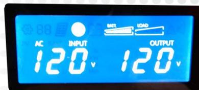
LCD display indicates input voltage, output voltage, load level, battery capacity, operation mode, and alarm conditions.
