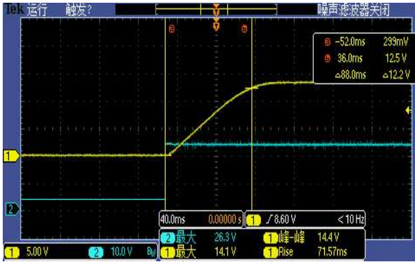
Figure 6, Output voltage established (Iout = 20A)
